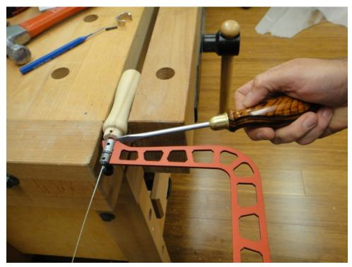
3. Loosen frame attachment hardware, position new handle and tighten set screws (Note: The Titanium saw frames have a slight variation in thickness. You may need to file the inside of the slot of the brass ferrule slightly to achieve proper fit.)
